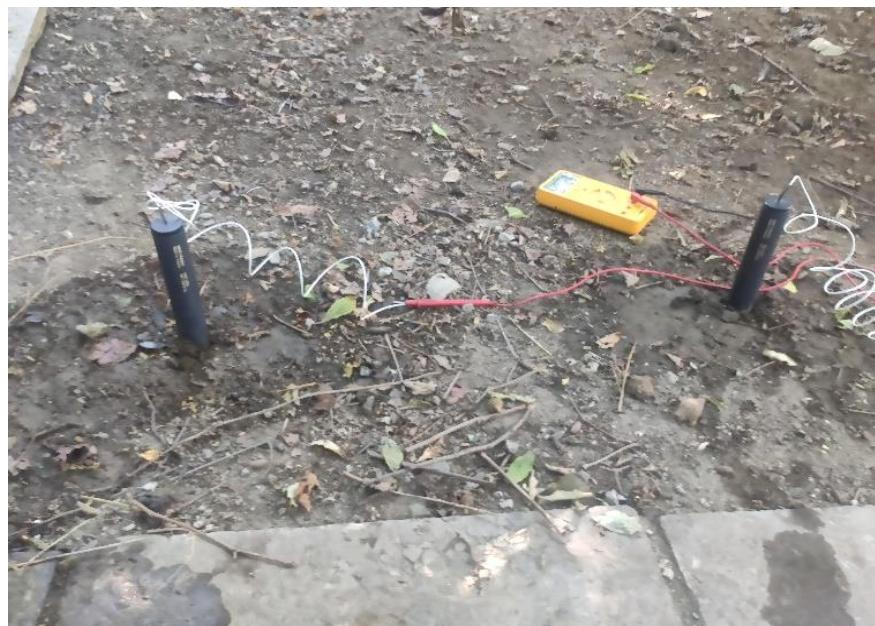
Fig. 6. Non-polarizable electrodes PMS 9000
