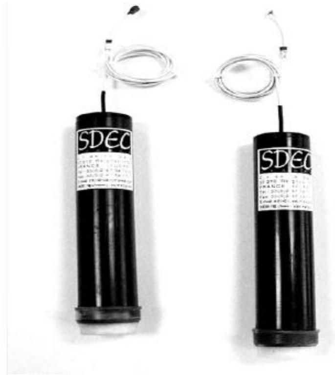
Fig. 2. Dry unpolarizable electrodes for self potentials measurement - PMS 9000
