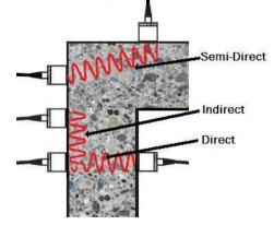
**Direct transmission:** Optimal configuration with maximum signal amplitude. The most accurate method for determining pulse velocity.
