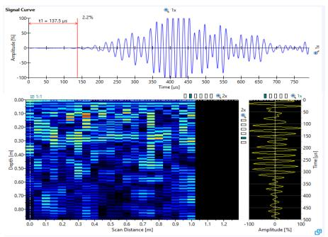
Fig.2. Ultrasound waveform (upper) and tomographic (lower) recordings.
