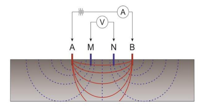
Fig.1. Schlumberger method of vertical electrical sounding
