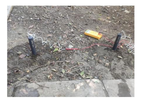
Fig. 6. Non-polarizable electrodes PMS 9000
