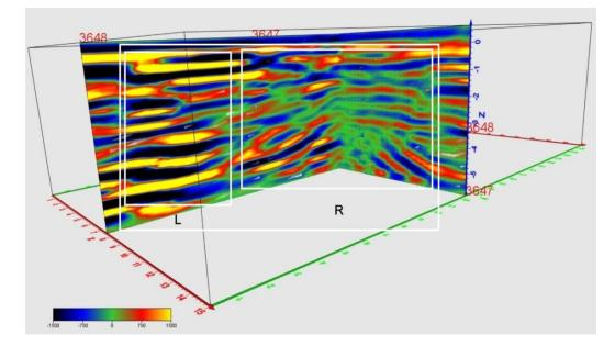
Fig. 8. 3D radio image created using profiles 5a and 5b radargrams. The lengths of the profiles are measured along the axes: Prof-5a length 15 m and Prof-5b - 25 m.
