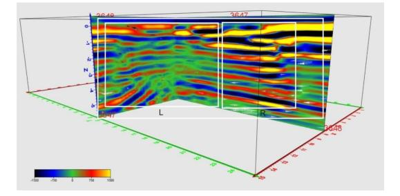
Fig.7. 3D radio image created with profile 5a and profile 5b radargrams. Profile lengths are measured along the Prof-5a axes at -15m, and Prof-5b at -25m. It consists of a "rear" file 3647 and a "rear" file 3648.
