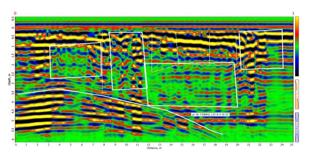
Fig. 4. GPR-section (profile 5b-3648) with a depth of 6 m and a length of 25 m, made by the Zond-12e georadar with a standard 150 MHz dipole antenna.
