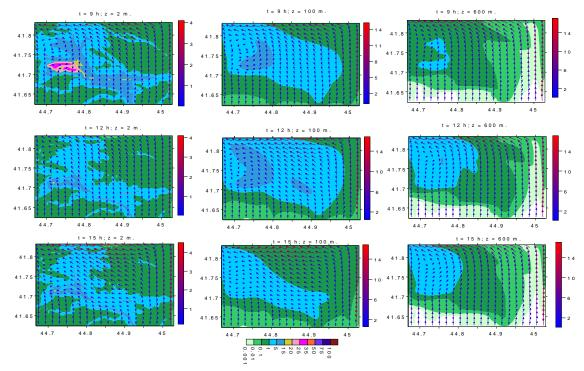
Fig. 5. Wind velocity (m/sec) and PM2.5 concentration (mcg/m<sup>3</sup>) fields in summer, in the surface and boundary layers of the atmosphere, when t = 9, 12, and 15 h.
