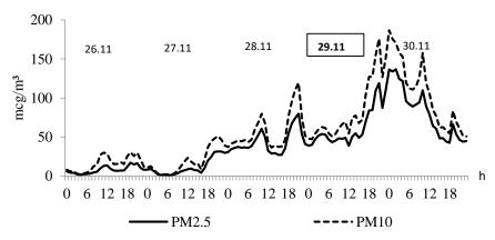
Fig. 2. Hourly motion of PM2.5 and PM10 concentrations on November 26-30, 2020 at observation point of monitoring situated at Tsereteli Avenue.
