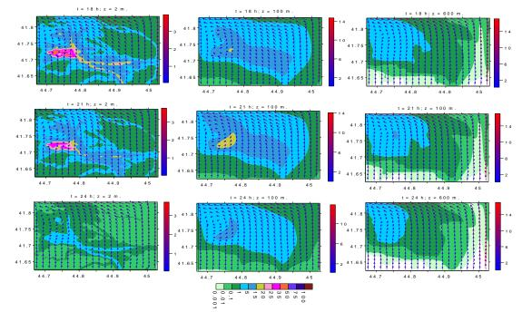
Fig. 6. Wind velocity (m/sec) and PM2.5 concentration (mkg/m<sup>3</sup>) fields in summer, in the surface and boundary layers of the atmosphere, when t = 18, 21, and 24 h.
