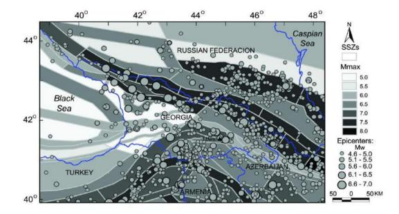
Fig. 8. ASSs maps of the investigated region, differentiated by  $M_{\text{max}}$ : (a) for ASSs Model 1. (b) for ASSs Model 2.
