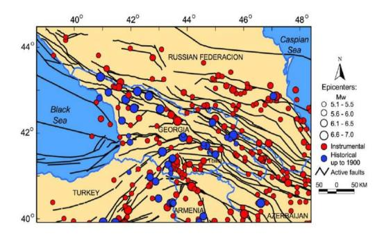
Fig. 3. Seismotectonic map: active faults, from Adamia et al. [1] and from Danciu et al. [5] and seismicity with  $M_W>5$  for Georgia and the regions around it (Zare et al., [19]; Varazanashvili et al., [15]).
