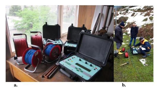
Fig.3. a) Earth Resistivity Meter PASI 16GL-N, b) measurement process.
