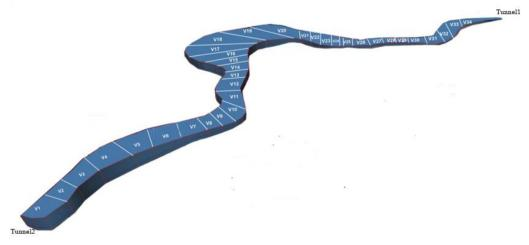
Fig.4. Temporary water reservoir model to calculate its volume
